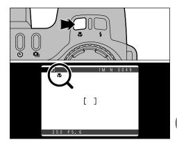
When you press the "\"" button, the "\"" icon appears on the screen and the camera is in Macro mode. Press the "\"" button again to cancel Macro mode.
